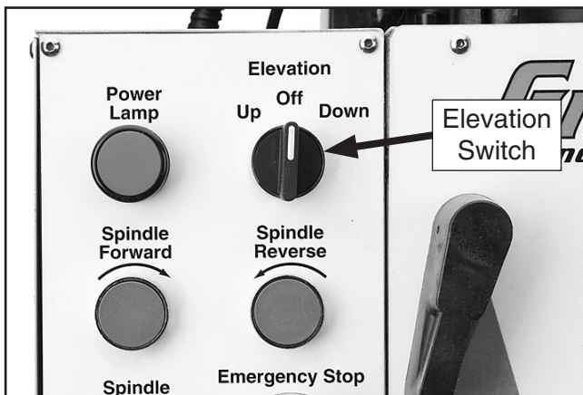
Figure 14. Elevation switch that controls motorized head travel.
